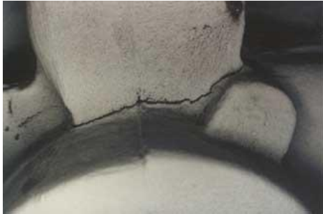
Figure: Crack in casting
